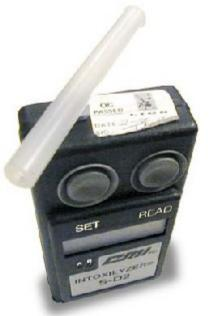
Police officers use portable breath-testing machines like this one to find out if a driver has a blood alcohol level above the legal limit.
